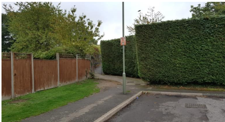
The railway bridge between Robin Way and Yew Tree Drive has a concealed entrance, no dropped kerb and is, again, extremely narrow for cyclists and pedestrians, despite being the only link between Stoughton and Bellfields north of Stoughton Road. Improvements here would need to focus on creating a more open and visible bridge crossing with clear lines of sight, as well as increasing the width of the bridge and approaches.
