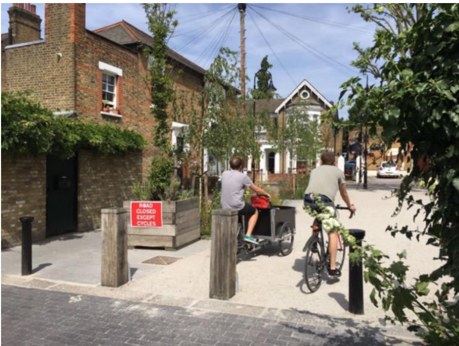
Modal filters can also be designed as a pocket park, providing benefits to the local community and improving the neighbourhood while also restricting vehicle through traffic. Modal filters can therefore be used to provide additional services to communities such spaces to play, green spaces, or places for businesses to utilise (such as space for pavement cafes or coffee carts).
